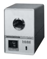
The black body furnace for medium temperature range is used for comparison calibration by utilizing a fixed-point calibrated  $0.90\,\mu\text{m}$  silicon monochromatic radiation thermometer as the standard thermometer, and the black body furnace for low temperature is used for calibration by utilizing a optional built-in platinum resistance thermometer as the standard thermometer.
