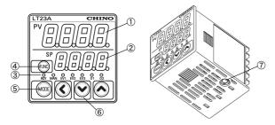
①Upper display: Displays PV values (preset temperature,etc) or
