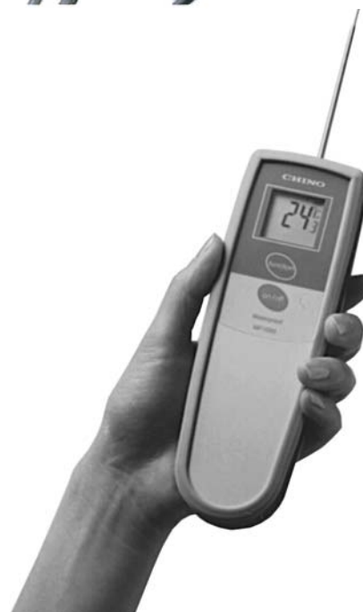
Temperature measurement by fitting the sensor to the backside of the thermometer
